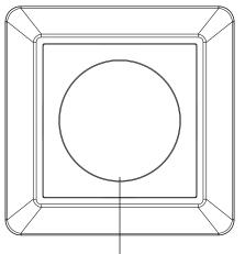
Rotary knob, short press to turn on/off, rotate clockwise to increase brightness, rotate counterclockwise to decrease brightness
