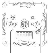
"Reset" Key: for Z-Wave network inclusion or exclusion, or factory reset the device
