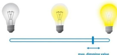
**Parameter no. 65 – Dimming time (soft on/off)**
