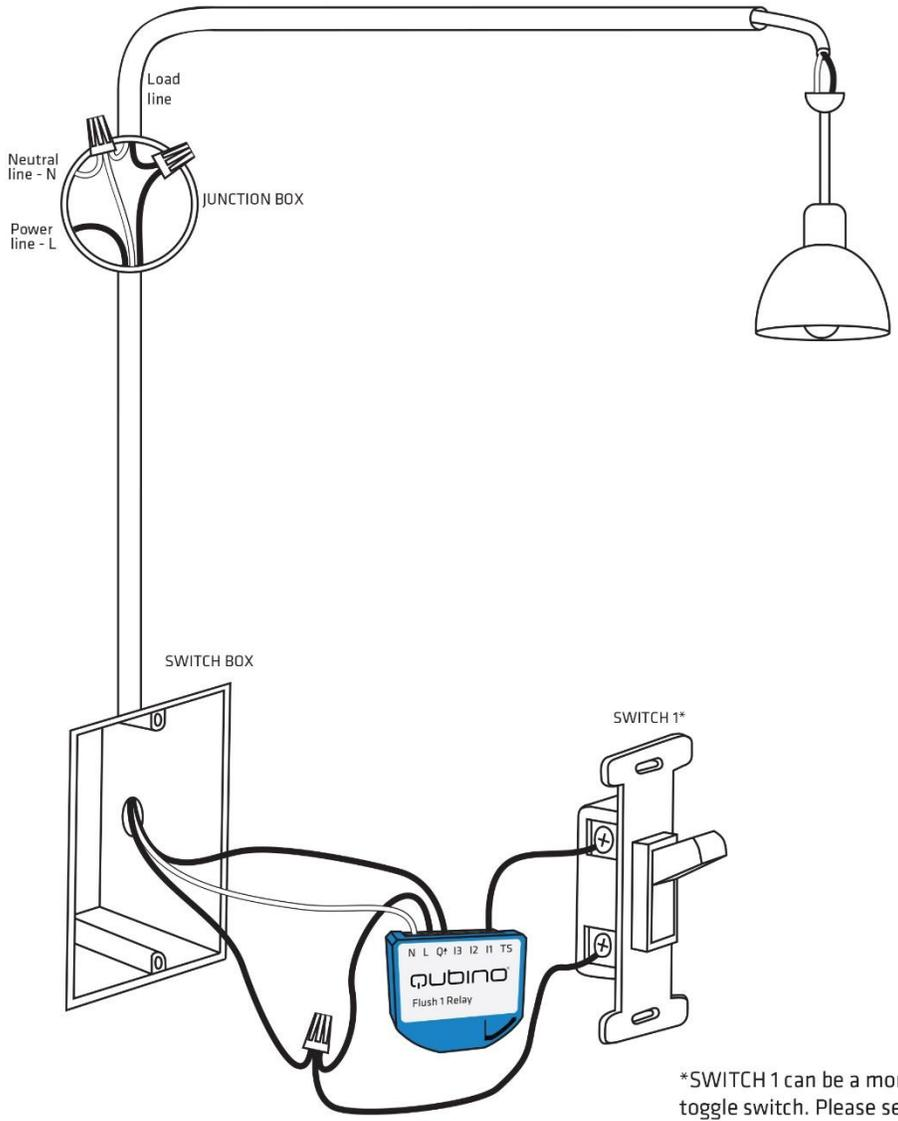
\*SWITCH 1 can be a momentary switch or a toggle switch. Please set parameter 1 to value 0 when connecting to a momentary switch. Set parameter 1 to value 1 when connecting to an on/off toggle switch (default setting). Please see the Configuration Parameters chapter for more information about advanced parameter settings.
