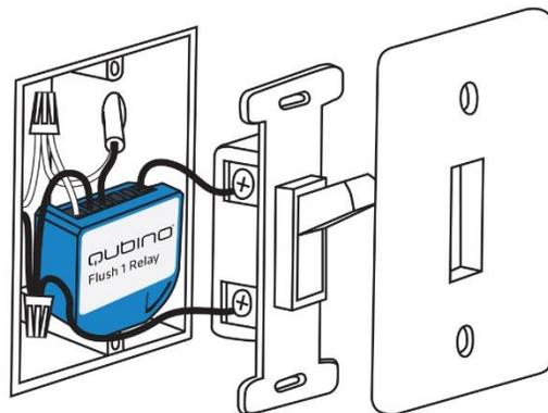
INSTALLATION WITH ON/OFF SWITCH AND SCENE SWITCHES:
