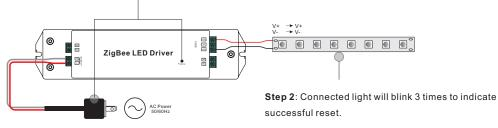
Note: 1) If the device is already at factory default setting, there is no indication when factory reset again . 2) All configuration parameters will be reset after the device is reset or removed from the network.
