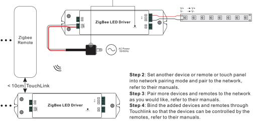
Note: 1) Each added device can link and be controlled by max. 30 added remotes.
