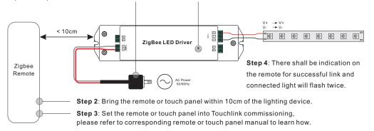
Note: 1) Directly TouchLink (both not added to a ZigBee network), each device can link with 1 remote. 2) TouchLink after both added to a ZigBee network, each device can link with max. 30 remotes. 3) For Hue Bridge & Amazon Echo Plus, add remote and device to network first then TouchLink. 4) After TouchLink, the device can be controlled by the linked remotes.
