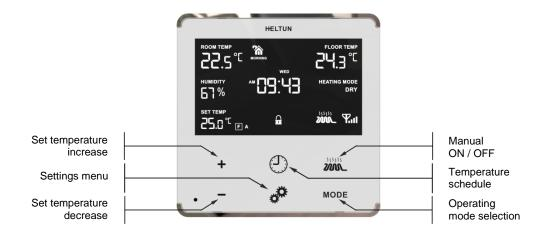
The Plus "+" button will increase Set Point temperature by 0.5°C with each touch. The Minus "-" button will decrease Set Point temperature by the same 0.5°C. The Set Point temperature is displayed in the bottom left corner of the LCD display under "SET TEMP."
