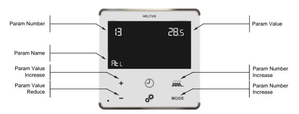
To scroll through the menu, press or hold the Heating Element button to go up and the "**MODE**" button to go down. To change the Parameter value, press or hold the Plus "+" or Minus "–" buttons.
